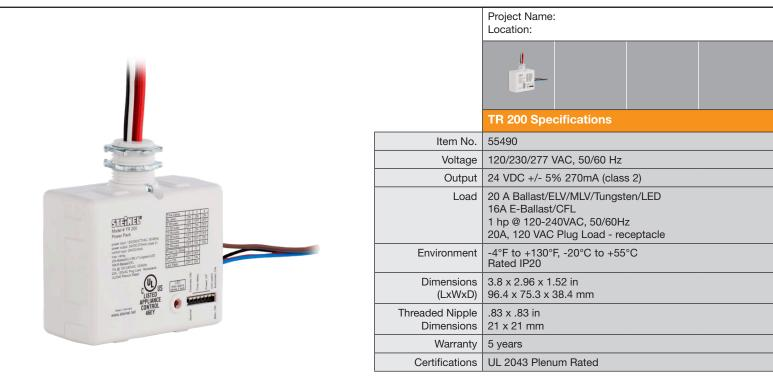
The TR 200 is a full-featured super duty lighting and plug load power pack that provides power to STEINEL low voltage occupancy sensors and other control devices. The power packs switch the load(s) on and off in response to signals from control inputs.
