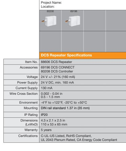
The DCS Repeater adds mA power supply to the Dataline allowing for additional sensors and switches to be added to STEINEL America's DCS or DCS Connect. This saves the cost of purchasing and installing additional DCS or DCS Connects on a job that simply needs more components.
